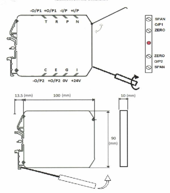
No tools are required when fitting a unit to a DIN rail. The moulded lugs at the base are simply hooked over one edge of the rail and, when the unit is pressed firmly home, it will latch into place and be securely retained by a spring-loaded clip. A screwdriver should be used when removing the unit from a rail. It should be used to ease back the clip, allowing the unit to be unhooked from the rail.
