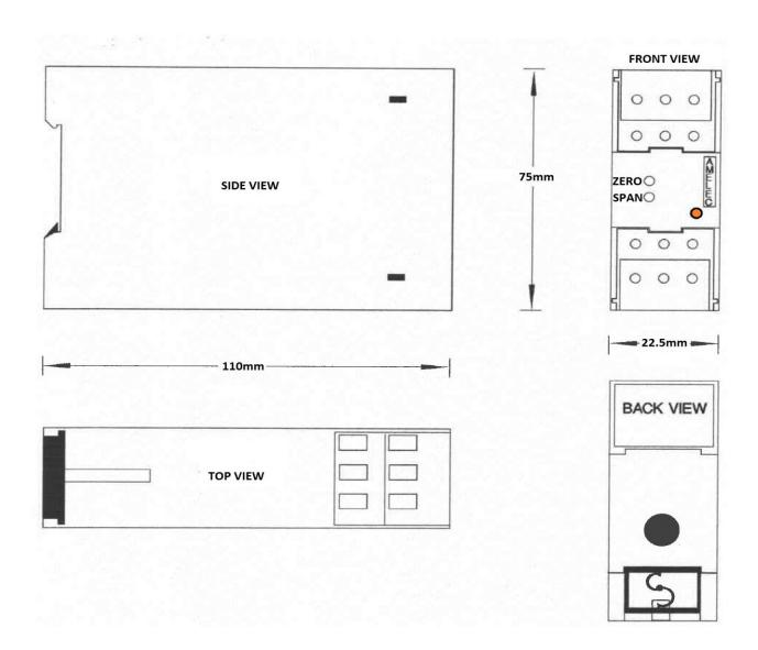
The enclosure material is Polyamide (PA), Nylon. UL94 V-2. Suitable for TS35 Top-Hat Rail mounting.
