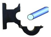
3. Screw the split-core back into closed position
