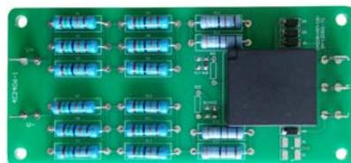
Closed loop voltage sensor based on the principle of Hall-effect.
