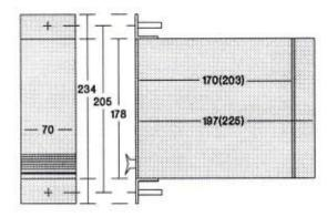
A 65mm wide by 190mm high aperture must be cut in the front panel with 6mm fixing holes above and below. The brackets and front panel are wider than the aperture to obscure any cut edges.
