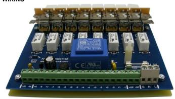
Screw terminal, 12 - 26 AWG / 250VDC / 10A
