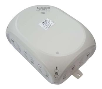
IP69 rated weatherproof enclosure suitable for outdoor installations. It is resistant to UV radiation and is protected against rain and saltwater, as well as being temperature and impact resistant. This junction box is ideally suited to offshore applications.
