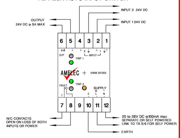
TRIP 1 / 2, 15 TURN POTENTIOMETER. RANGE 20 - 25Vdc. Factory set at 21V.
