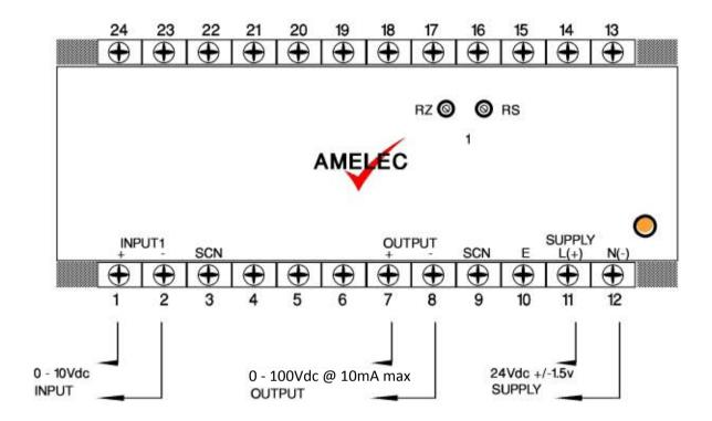
ZERO / SPAN ADJUSTMENT +/-10%
