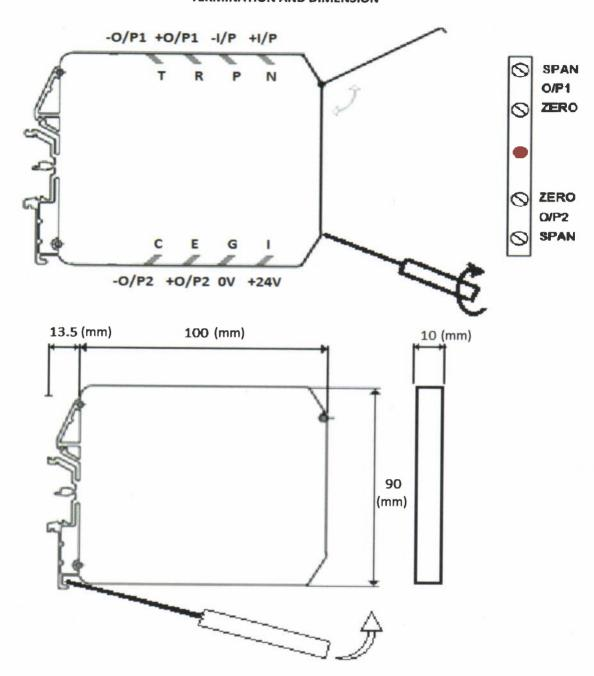
No tools are required when fitting a unit to a DIN rail. The moulded lugs at the base are simply hooked over one edge of the rail and, when the unit is pressed firmly home, it will latch into place and be securely retained by a spring-loaded clip. A screwdriver should be used when removing the unit from a rail. It should be used to ease back the clip, allowing the unit to be unhooked from the rail.
