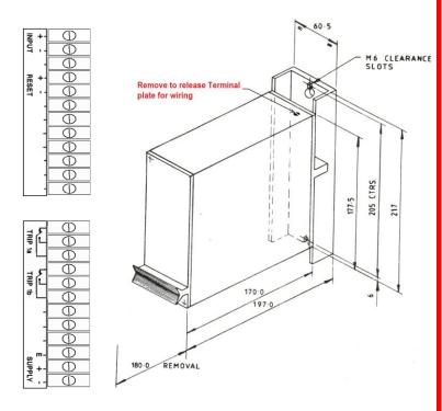
The terminal plate can be removed from the case by removing the M4 hexagon headed screw at the top rear of the case, hinging the case downwards and unhooking it from the fixed peg at the lower rear of the terminal plate assembly. This exposes the terminal plate for wiring.
