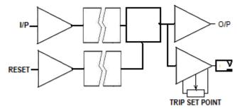
Basic function of the unit is to monitor the input and count the number pulses. The total of the count is compared against the trip set point. When the total exceeds the set point, the relay is tripped. The counter can be remotely reset by a pulse.
